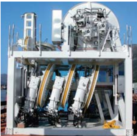
Winches with secondary drive technology can be used down to a depth of 4,000 meters.
