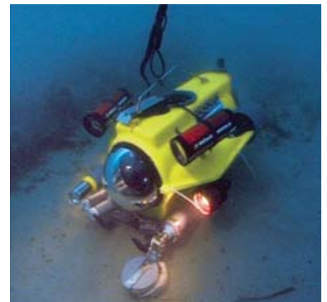
A remote-controlled submarine robot helps to place loads on the seabed.
